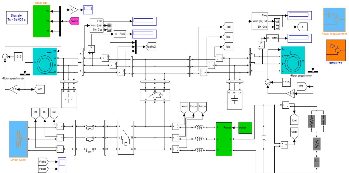
Fig. 2 MAT LAB simulink model of the parallel operation of isolated asynchronous generators
