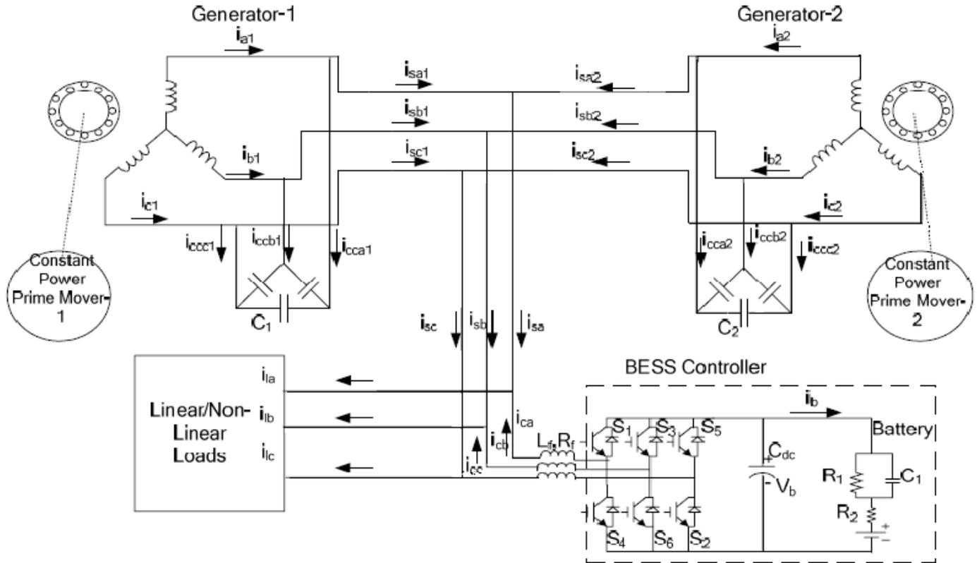
Fig. 1. Schematic diagram of parallel operated isolated asynchronous generators
