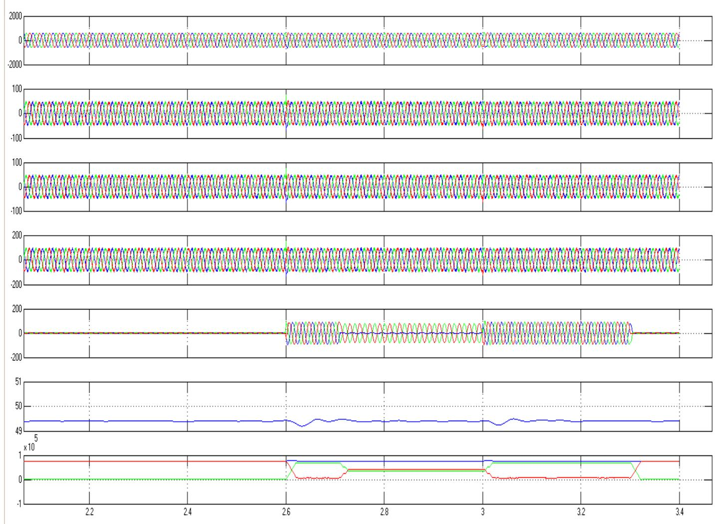
Fig. 3 simulation results of generation of voltage (Vsabc), generation of current 1 (Igab1), generation of current 2 (Igab2), source current (Isabc), load current (Iabc1), frequency (f), load power (p) respectively.
