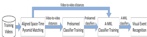
Fig.2. The flowchart visual event recognition framework. It consists of an aligned space-time pyramid matching method that effectively measures the distances between two video clips and a transfer learning method that effectively copes with the considerable variation in feature distributions between the web videos and consumer videos.
