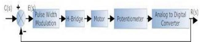
Fig.3 Simple closed loop in frequency domain
