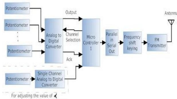
Fig.8 Wireless Transmitter
