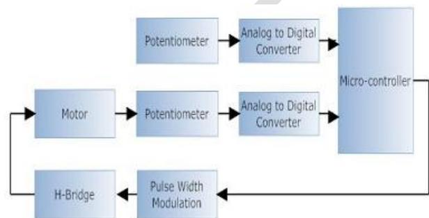
Fig.2 Simple closed loop system
