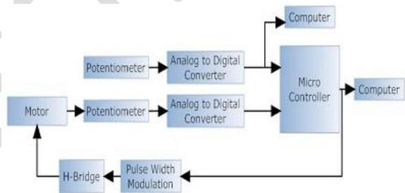
Fig.12 Closed loop system
