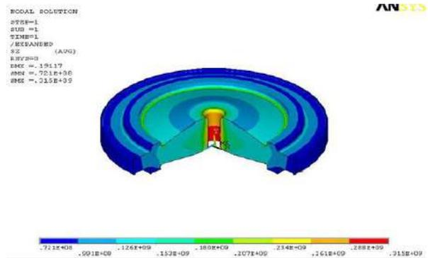
Fig 4: Stress distribution along z-direction for rotational load
