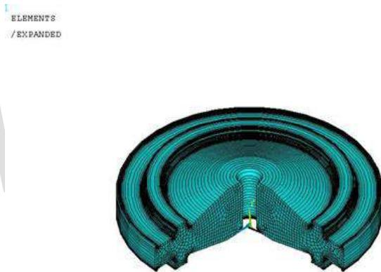
Fig 2: Mesh model of gas turbine rotor wheel
