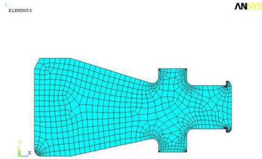
Fig 1: Mesh model of gas turbine rotor wheel cross-section
