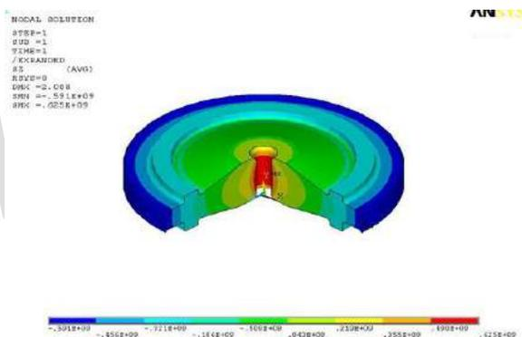
Fig 6: Thermal gradients of gas turbine rotor wheel
