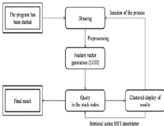
Fig:1 The data flow model of system from user point of view
