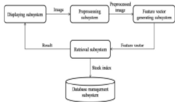
Fig. 1. The global structure of the system.
